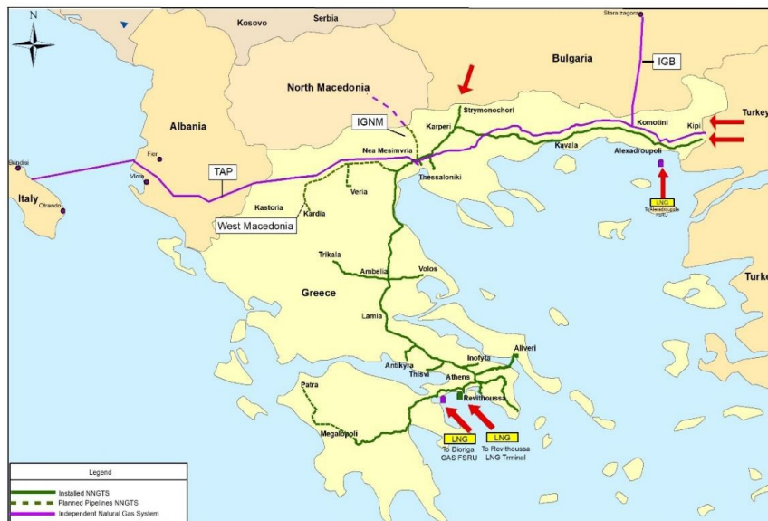
Figure 2: Map of the Greek National NG Transmission Grid and its connections
